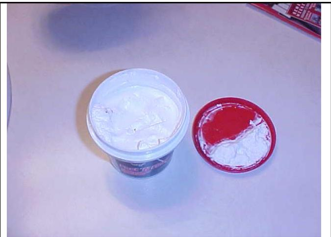
The recommended way to repair stress cracks in walls and ceilings is to use lightweight spackling.
